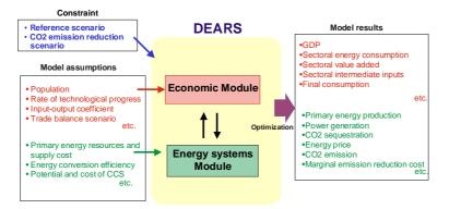
Figure 1 : Inputs and outputs of DEARS
