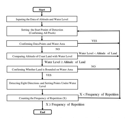
Figure 1 Flow Chart of level flood method
