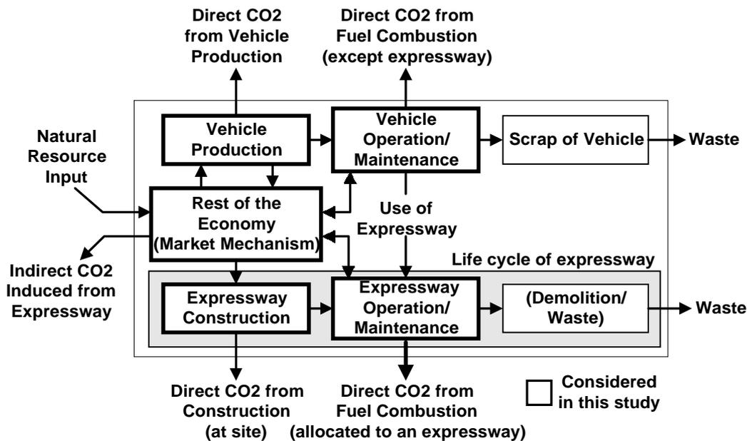
Fig. 2.1 Framework of the Analysis of Life Cycle Emission of Expressway
